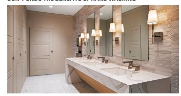
Use offset drains in sinks so that water falls onto the bottom surface of the sink, rather than into the drain which can cause bacteria that went down the drain to splash back up at the user.
